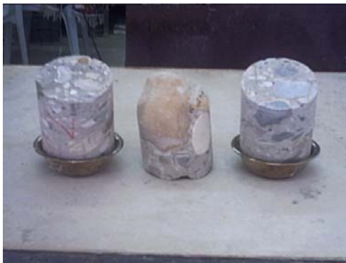
(c) Core Samples from Concrete showing type of aggregates used. (Shifa Hospital)
